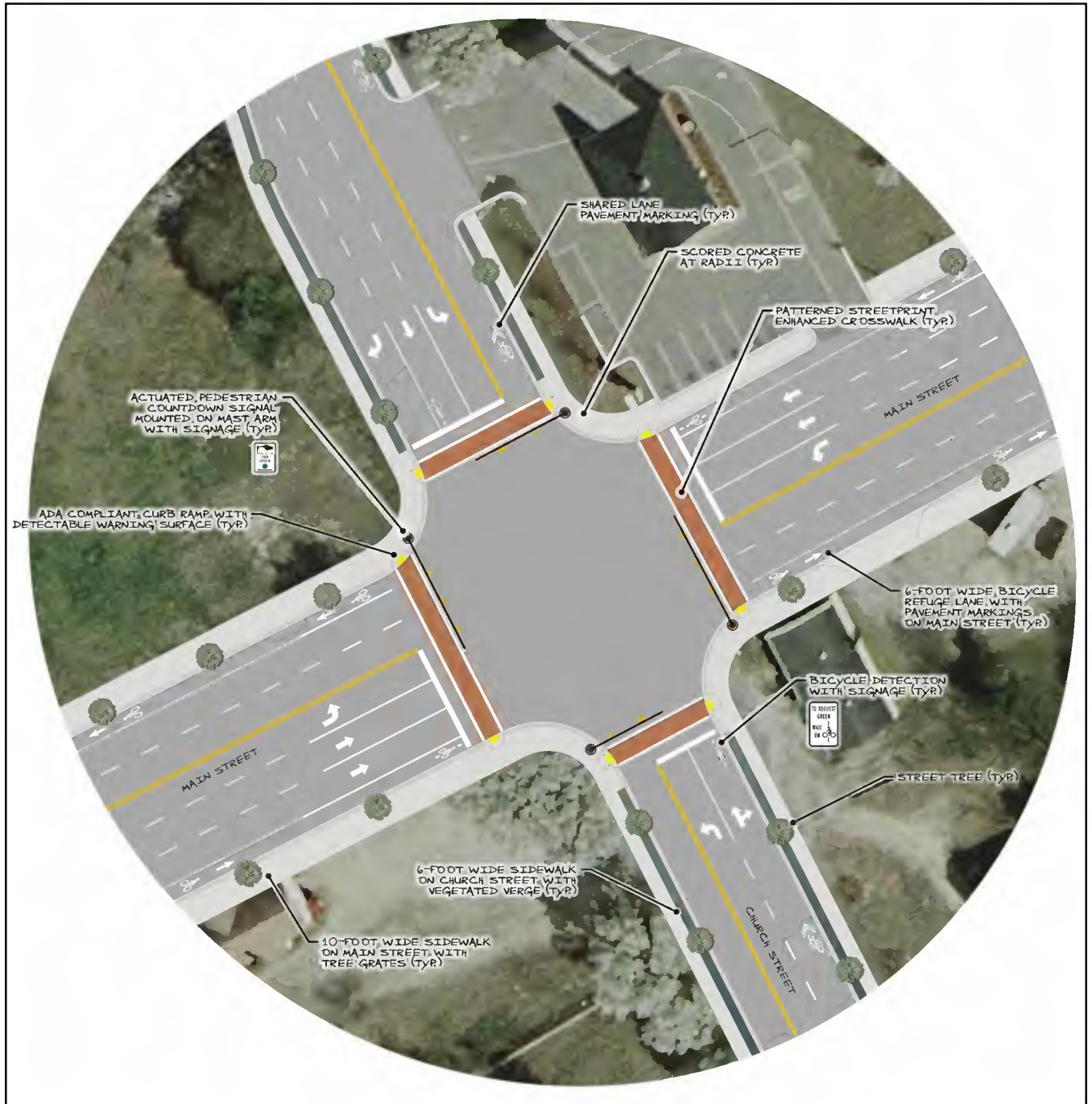
Figure 4.3-1: Main Street/Church Street Intersection Schematic Design
