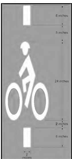
Bicycle Detection Marking and Signage (Source: MUTCD)
