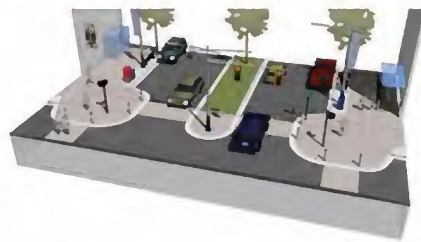
Traffic Calming Measures Small curb radius, raised intersection, demarcated pedestrian crossing, curb bulb-outs, prioritized signalization.
