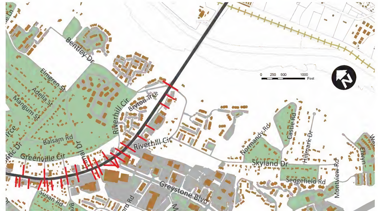
Figure 19: Existing Driveways - Southern Portion
